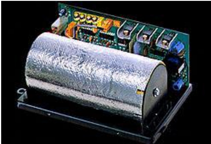
Fig. 4: Outside construction of gas-rate gyro sensor.
